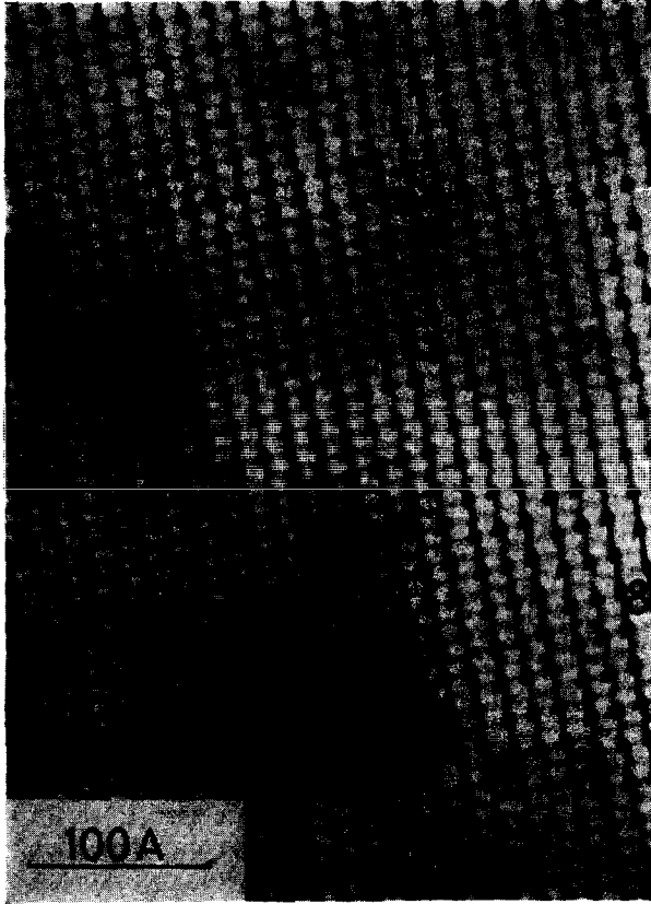
FIG. 9a. Crystal fragment containing \text{Me}_{25}\text{X}_{62} (C-rows) and lamellae of \text{Me}_{28}\text{X}_{70} (D-rows, numbered 1-8) D-rows 4 and 5 move laterally via an area of dense contrast.
